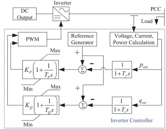
Fig. 14. Power-electronic-dominant microgrid equivalent model.
