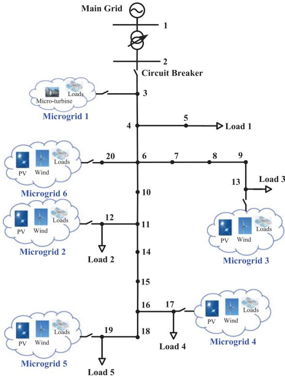
Fig. 2. A typical networked microgrids system.
